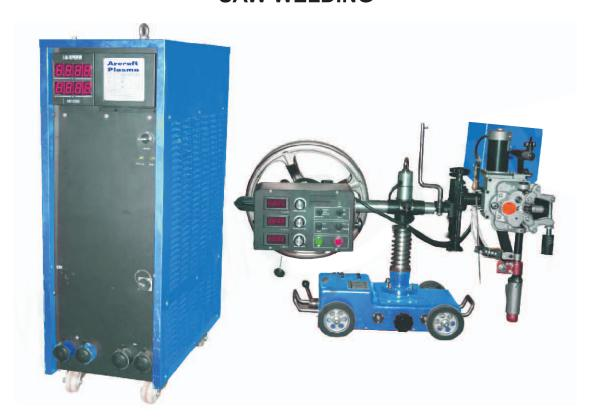
Submerged arc welding (SAW) is a semi-automatic or fully automatic consumable electrode arc process in which the arc is protected by a granular, fusible flux which blankets the weld puddle and surrounds the base metal to protect it from the atmosphere.
