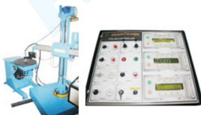
Column & Boom With Process Control Panel
