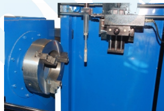
Hollow Barrel Chuck & Oscillation System
