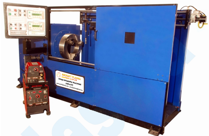
Hardbanding Machine with Power Source
