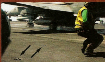
Fig. 9 — Explosion welded aircraft tie-down fittings welded into aluminum aircraft carrier decks never need replacing. See lead photo.
