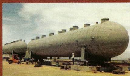
Fig. 11 — This large high-pressure autoclave is used to leach laterite nickel ore in hot sulfuric acid. The vessel is constructed from corrosion-resistant titanium clad to 4-in.-thick steel for strength. (Courtesy of Dynamic Materials Corp., Boulder, Colo.)
