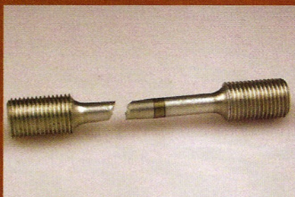
Fig. 4 — Tensile testing of this Al-stainless steel-Al specimen displays the strength of the explosion welds exceeded that of the aluminum.
