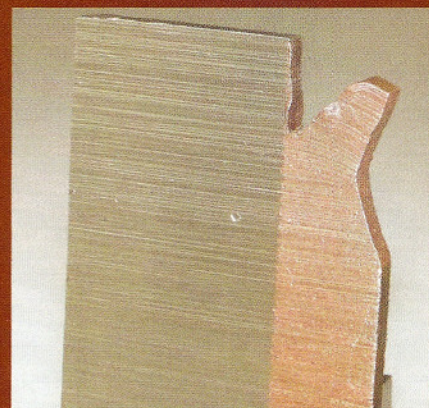
Fig. 5 — The chisel test showed no separation at the weld in this stainless steel-copper specimen.
