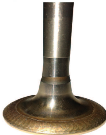
Valve stem hardfaced with PTA
