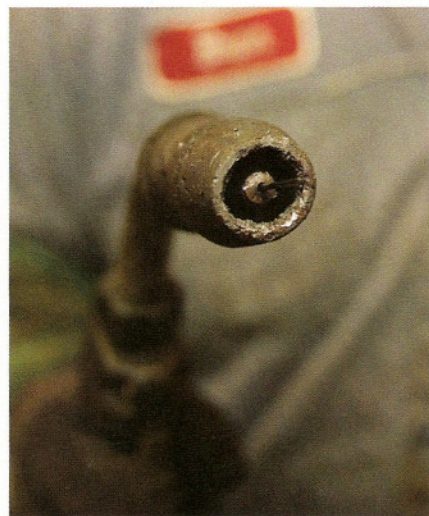
Fig. 2 — As seen here, GMAW gun consumables are exposed to a lot of abuse during the normal course of welding. Regularly maintaining these products can extend their life and increase a company's productivity.
