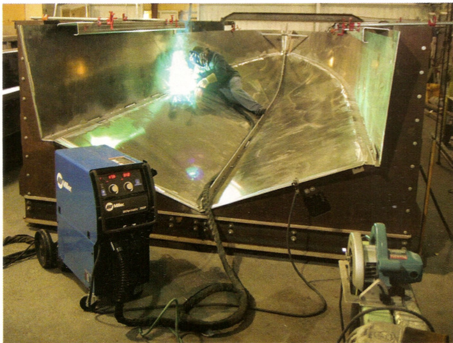
Fig. 2 — With GMAW-P, operators at Metal Shark Aluminum Boats, Jeanerette, La., can make long welds without having ribs in place because the welding process does not cause any heat-related distortion.
