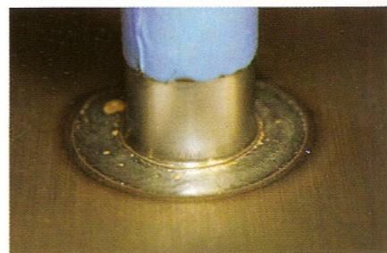
Fig. 3 — By switching to a GMAW-P system for its mild steel, welded barbells, Iron Grip Barbell Co., Santa Ana, Calif., was able to eliminate the need to apply antisplatter, while increasing productivity by 16%.
