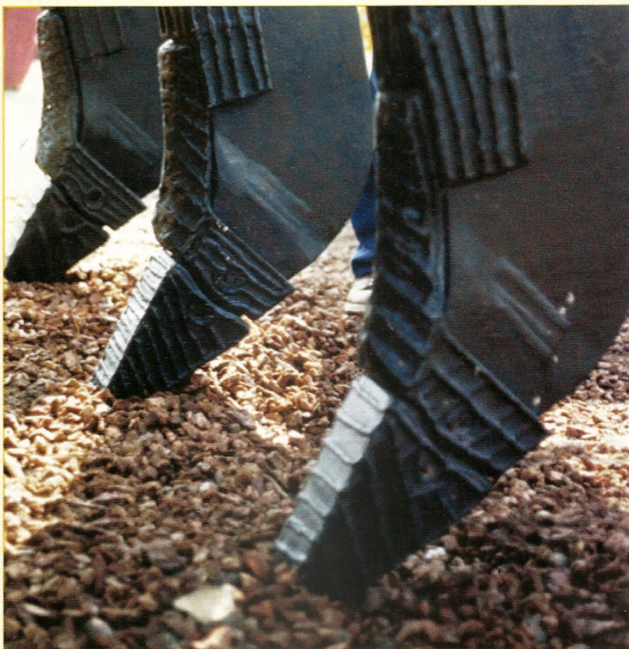
Fig. 4 — Stringer beads are weld beads that run parallel to one another and are suitable for certain buckets used on earthmoving or heavy construction equipment.
