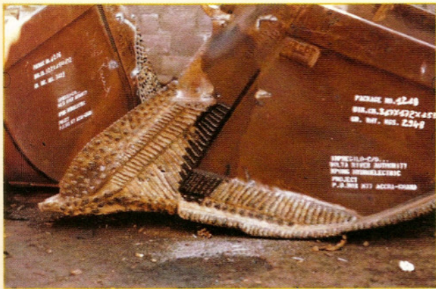
Fig. 2 — The herringbone pattern, shown on the side of this bucket, is formed by laying weld beads at varying angles.
