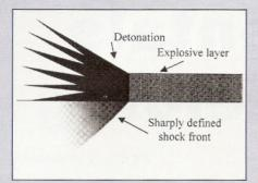
Fig. 1 — A shock wave develops when the sonic velocity of the explosive is greater than 120% of the sonic velocity of the faster metal.
