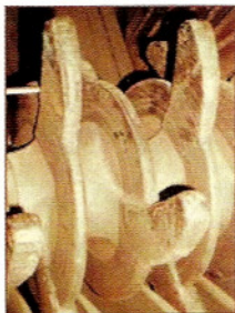
Fig. 8 — Sinter crusher blades hardfaced with a composition that exchanges molybdenum with chromium.
